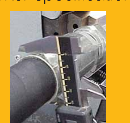
Measurement 2 at the beginning and the end of the ferrule (displaced by 90°)
